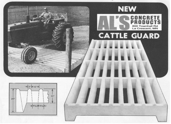
Al's Concrete cattle guards are heavily reinforced and precast in one piece to insure a lifetime of maintenance free operation. Both sizes support the heaviest machinery load and use a bottom flow through design for water flowage. Available in 12 and 16 foot lengths.
